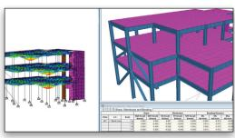
Generate analytical models directly from the engineer's physical model with STAAD.
