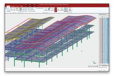
Physical modeling capabilities enable engineers to better participate in BIM workflows, automatically generating the analysis models for both simple and complex structural analysis.
